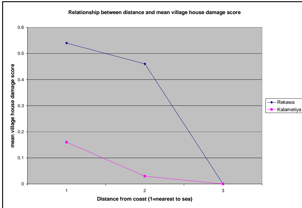
Figure 2. Relationship between distance and mean village house damage score
